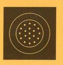
The Selas RSA Refrak Screen Burner is a sealedin tunnel burner with superior flame retention and combustion characteristics. The RSA's large, perforated refractory screen distributes the air/gas fuel mixture uniformly within the tunnel, and assures complete combustion over an extremely wide throttling range.
