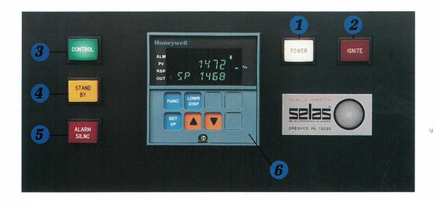
recision Combustion Monitoring and Control The Selas Raw-Gas Qual-O-Rimeter monitors and automatically corrects fuel gas quality to user requirements. The Q-O-R continuously burns a small sample of blended gas and instrument air in a thermally balanced combustion chamber. The temperature of the sample flame is affected by a change in the blend ratio.
