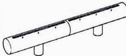
Multi-zone burner, internally partitioned
